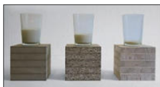
MDF 74 ml/dm 3 , Span 46 ml/dm 3 , SWL STAB 11 ml/dm 3
